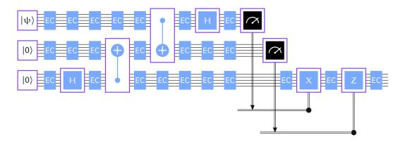
Suppose (for simplicity) that we use the 7-qubit Steane code, so our error corrections can correct for 1 error per code block.
