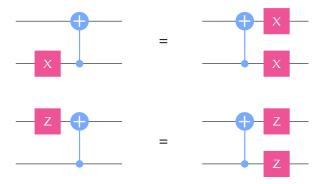
This can create correlated errors on two qubits. (Two-qubit gates can also be faulty, causing correlated errors on multiple qubits.)
