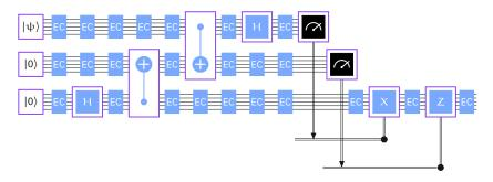
Some codes allow for *transversal* implementations of certain gates — meaning a tensor product of operations acting on a single qubit position within each code block.
